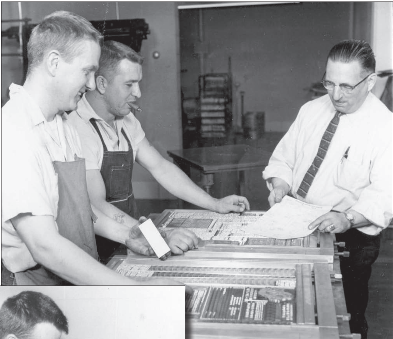
Above: Columns of news lines, headlines and ads are assembled in page form in the makeup area of the composing room. Norbert Kubisiak, left, and Earl Heineck, makeup men. Mechanical supt. Al Wenzlaff, right.
