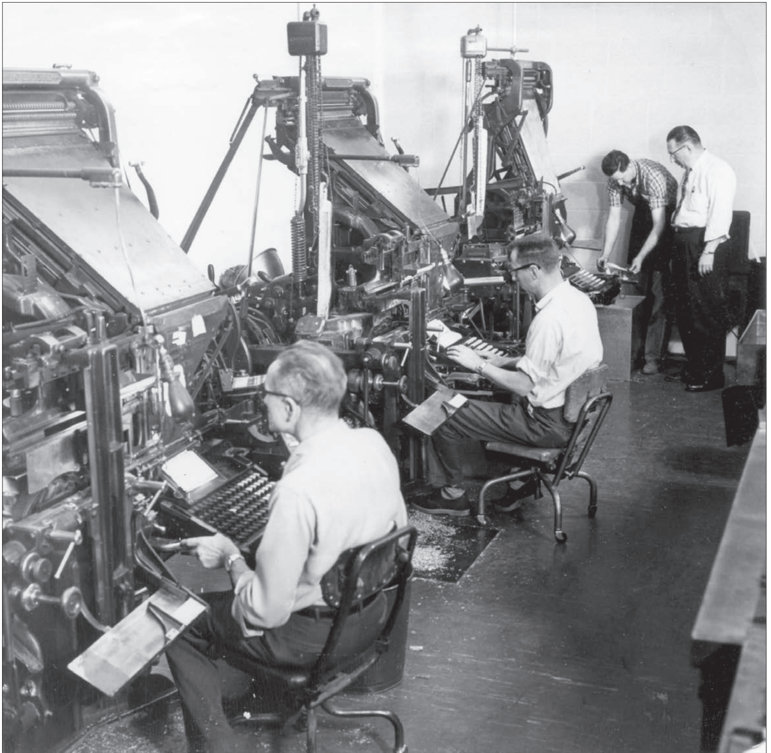
Above: Setting lines of type in the composing room. From left, Frank Niklaus, Charlie Bidwell. Clifford Forster and Al Wenzlaff, checking output of perforated paper tape fed through automated teletypesetter units. The high-tech perforations that magically sent the news from place to place originated in the Associated Press Bureau, Milwaukee.
