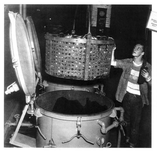
Photo by former *Tribune* photographer Don Krohn, shows what appears to be a Sampson Canning Co. worker removing a batch of peas or beans from a cooker.
