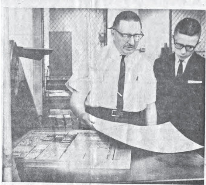
MAT ROLLER —To convert a flat page of type and illustrations into a curved plate which will fit a cylindrical press requires the preparation of a “page mat” from which the press plate can be cast. Mechanical Superintendent Al Wenzlaff is demonstrating this process for Wayne Martin.
