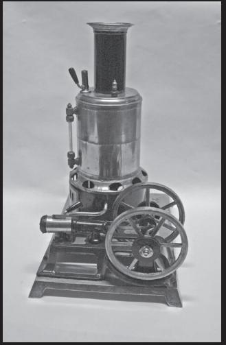
From Marshall's collection. Top left: Steam powered both miniature and full-size automobiles. Left above: Weeden classic engine from turn of century. A slide valve admits steam to the cylinder. Right: Vertical boiler with two flywheels. Facing page: Sterling hot air engine didn't use steam.
