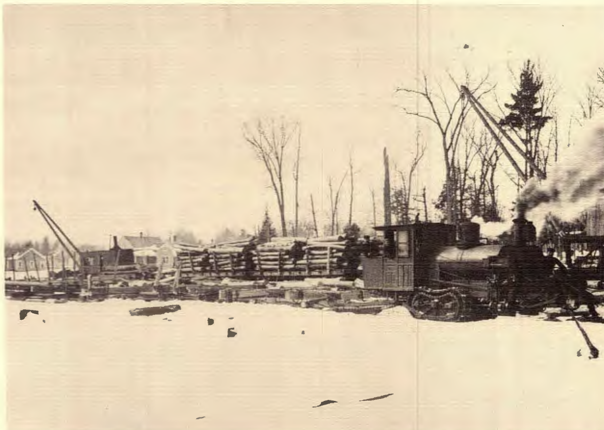
A Lombard steam hauler builds up a head of steam prior to hauling a train of empty sleighs into the woods. The crane, popular-
